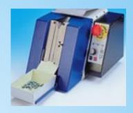
The TP/TC4 machine is designed to cut loose radial components. The speed and cutting lenght are adjustable. The machine stops when the front cover is removed. The lenght of the leads in origin must be L + 6 mm minimun.
