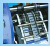
200240 body guide Max leght component body = 45 mm
