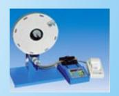
The County is a microcomputer based instrument which counts radial and axial components on tape. With the optional SMD adaptor it can also count SMD components. It counts in both directions (right or left). It is equipped with a divider from 1 to 19 and a TOTALIZER mode counting or PRESET mode, with an alarm that starts when the desired component number has been reached. Calibration test and self diagnostic procedure, last counting value and condition memory.
