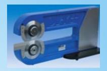
Manual machine suitable to separate pre-assembled Electronic Board. Precise, reliable and safe. The PCB is manually fed between the lower and upper blades using the scoring as reference. By pushing the board horizontally, the blade rotation starts offering a sharp and accurate cut. The blade height is adjustable depending on the thickness of the PCB.
