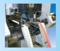
Olamef's knowledge and experience manufacturing forming machines are applied when designing this new line of equipment It helps to eliminate manually forming and inserting through hole components.
