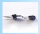
SP26.06 CUT AND "S" BEND FORM SUITABLE FOR FLAT LEADS
