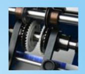
Minimum cutting lenght "B" =4,6mm and maximum lead "d" =0,8mm
